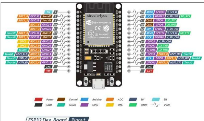
**GPIO Pins:** ESP32 Wroom32 DevKit has total 25 GPIOs out of that few pins are Input only Pins, Input Only Pins
